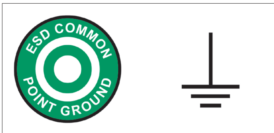
Figure 3: The common ground point symbol from ANSI S8.1 (at left) and the general earth (ground) terminal identification symbol from IEC 60417 (at right).
