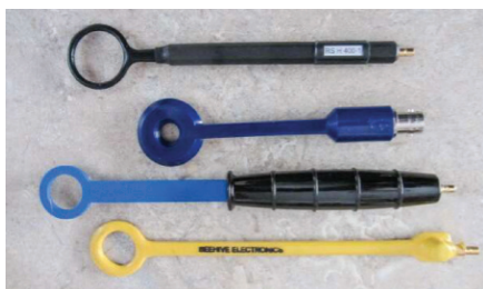
Figure 2: A variety of commercial H-field probes. Rohde & Schwarz, Com-Power, Tekbox and Beehive Electronics (top to bottom).
