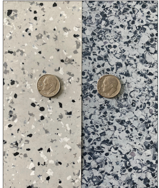
Figure 8: Low-density chip floor (on left) and high-density chip floor (right)
