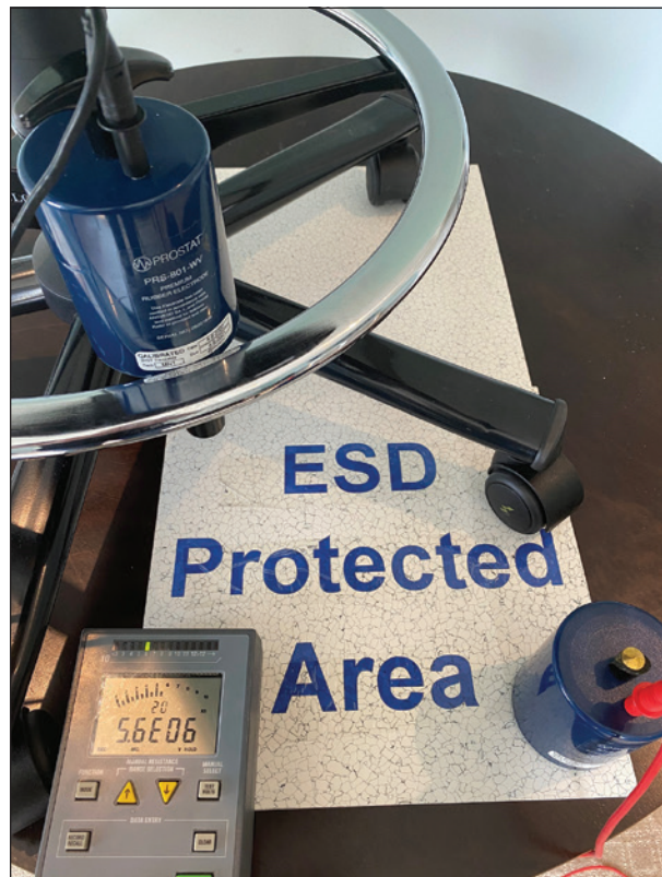
Figure 10: A conductive vein matrix ensures compliant grounding.
