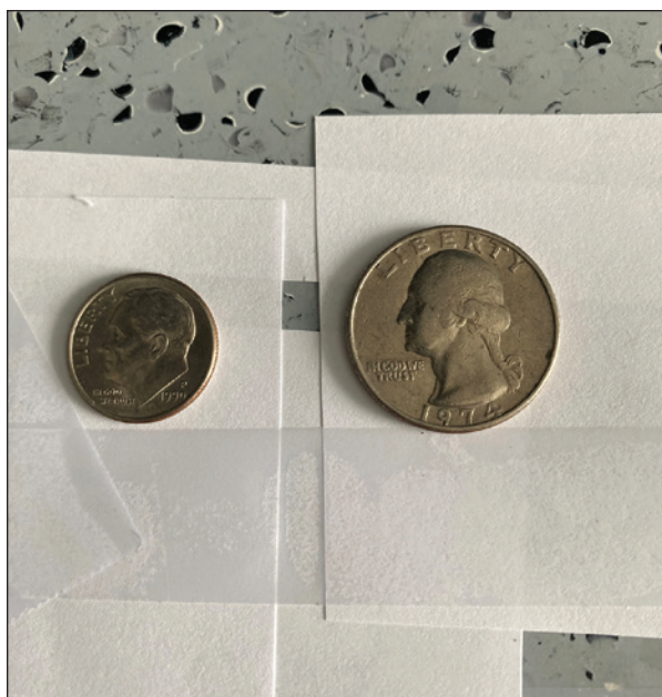
Figure 6: The solid grey area between the quarter and the dime represents the contact area of the caster and tile.
