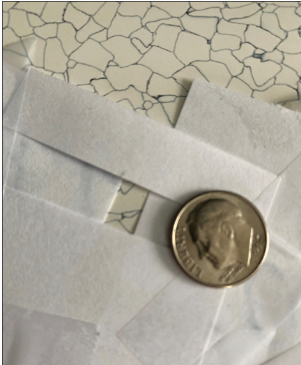
Figure 7: Contact area/patch of caster superimposed over conductive vein technology floor
