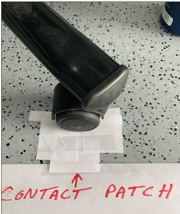
Figure 5: A space or void would show a contact area/patch between caster and tile.
