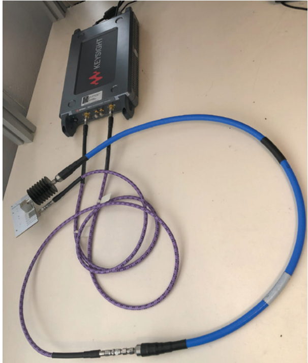
Figure 5: Test setup of the insertion loss measurements
