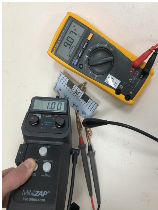
Figure 8: Verifying the ESD gun's voltage
