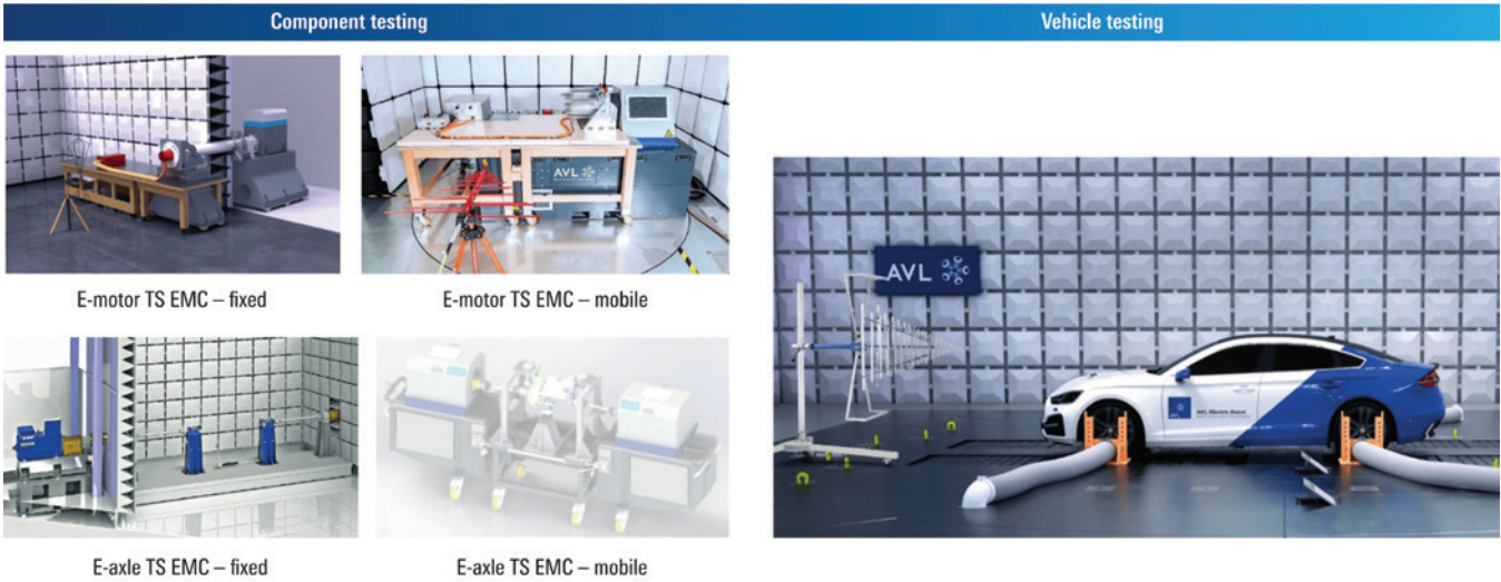
Figure 3: Full compliance test systems for powertrain components from hybrid vehicles and EV (left) and a full compliance test system for ICE vehicles, hybrids, BEVs and FCEV
