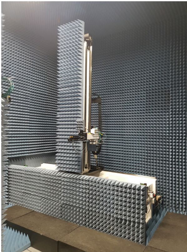
Figure 4: A planar near-field scanner showing the tower for the vertical scan resting on the horizontal stage for the horizontal motion of the probe
