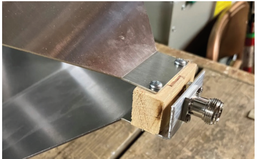
Figure 7: Parallel plate termination modification detail
