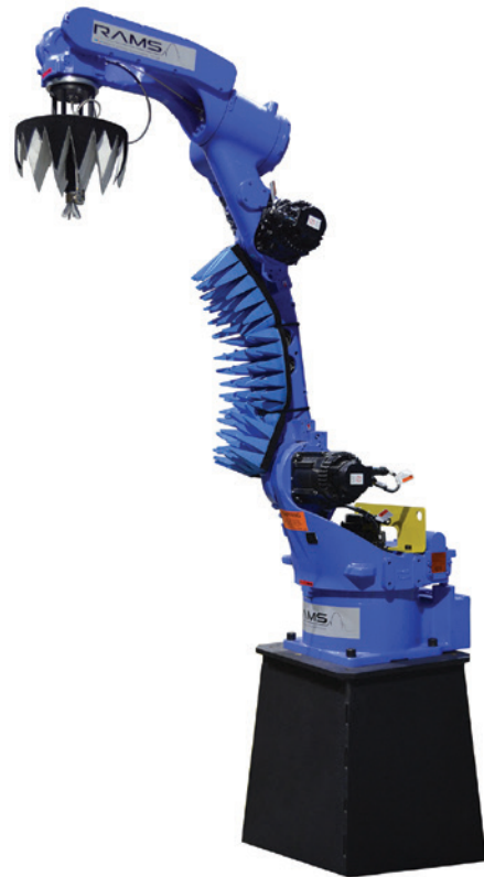
Figure 5: A robot arm-based near-field system that allows for non-canonical arbitrary surfaces to be measured
