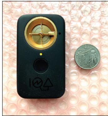
Figure 2: A miniature electric field mill configured as a wireless body voltage monitor (with a quarter for a sense of scale). The unit is 75 x 43 x 18mm in size, weighs 44g, and can run for 18 hours on a single battery charge.
