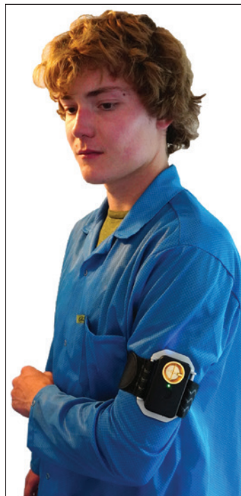
Figure 3: A person wearing a wireless body voltage monitor. The unit is worn over an ESD smock, with the sensor pointing outwards. The upper arm has a good combination of practicality, being close to the body core, while also unlikely to be obstructed by other body parts, and not being obtrusive.
