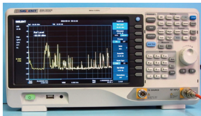
Figure 3: An example of an affordable spectrum analyzer usable for pre-compliance testing of conducted emissions.
