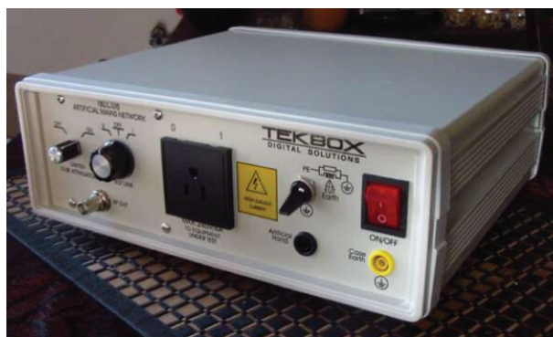
Figure 6: An affordable LISN. It has a switch that measures either line or neutral noise voltages and also includes a built-in 10 dB attenuator and transient protector.
