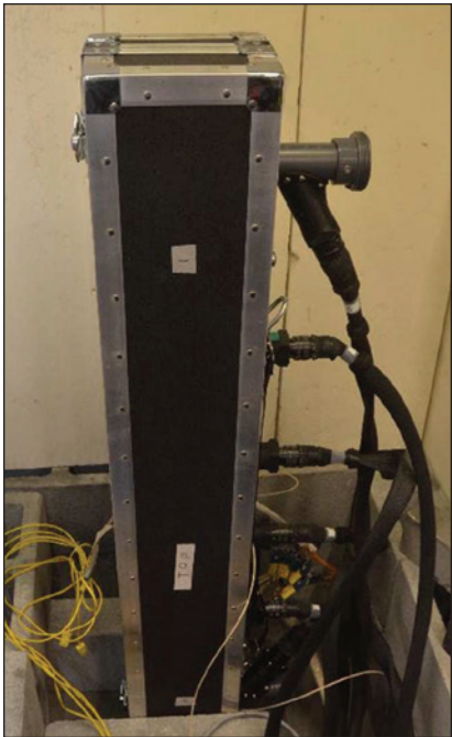
Figure 6: Photograph of an FTRC apparatus. View of the insulating casing utilized to enclose the calorimeter prior to each test.
