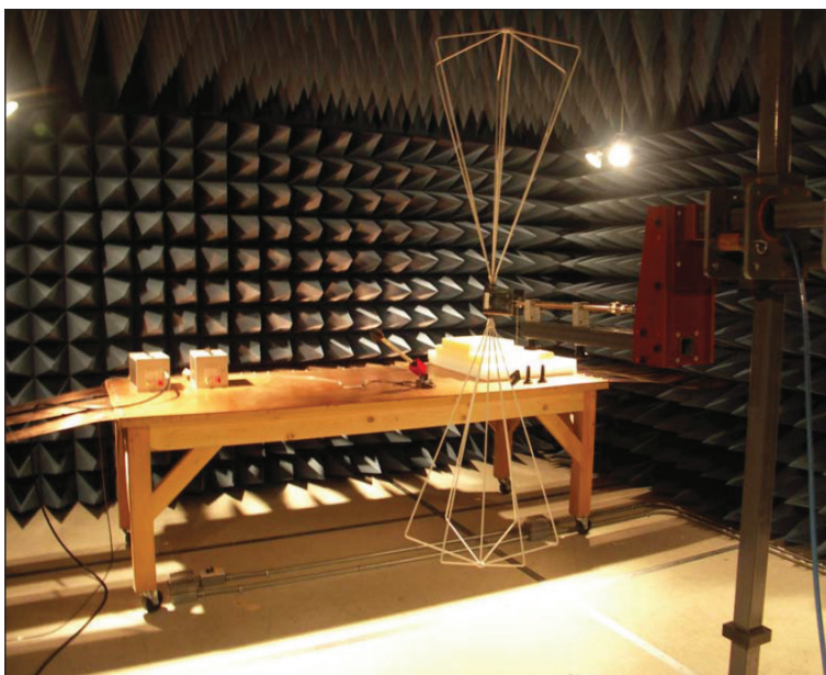
21 st century EMI test chamber. (Photo courtesy of Rohde & Schwarz.)
