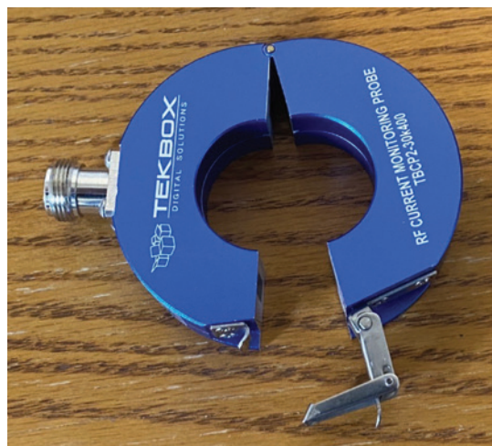
Figure 1: A typical RF current probe from Tekbox with useful frequency range of 30 kHz to 400 MHz (3dB bandwidth).
