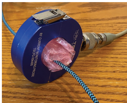
Figure 2: Using an RF current probe to measure the common mode currents on a USB cable.
