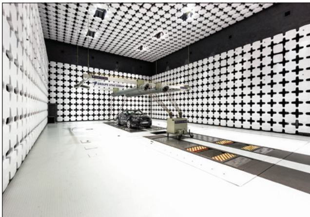
Figure 22: Automotive test chamber using polystyrene absorber (image courtesy of ETS-Lindgren)
