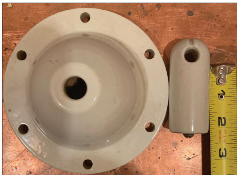
Figure 3: The circular ceramic is the fuselage penetration treatment for the unshielded antenna lead-in. It wasn't just the 5 kV transmit voltage driving the treatment, but also the high frequency requiring control of shunt capacity. Control of shunt capacity was provided within the aircraft by ceramic standoffs. The 2" distance between the base and the hole is the basis for the 2" (5 cm) standoff requirement in all subsequent EMI specifications and standards. (Photo courtesy of the Museum of EMC Antiquities.)
