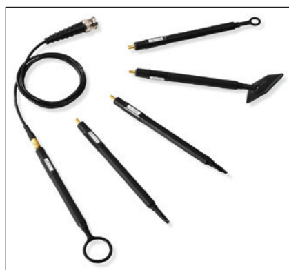
Figure 6: Typical near-field probes used in pre-compliance testing (Source: Rohde & Schwarz)
