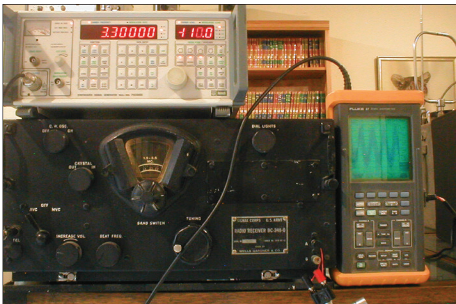
Figure 4: The author's unaltered BC-348Q radio, the specific radio model whose performance characteristics drove the emissions and susceptibility requirements in MIL-I-6181B below 20 MHz. The photo shows a noisy but audible response to a 1 kHz modulated radio frequency signal at a level of -3 dBuV. (Photo courtesy of the Museum of EMC Antiquities.)
