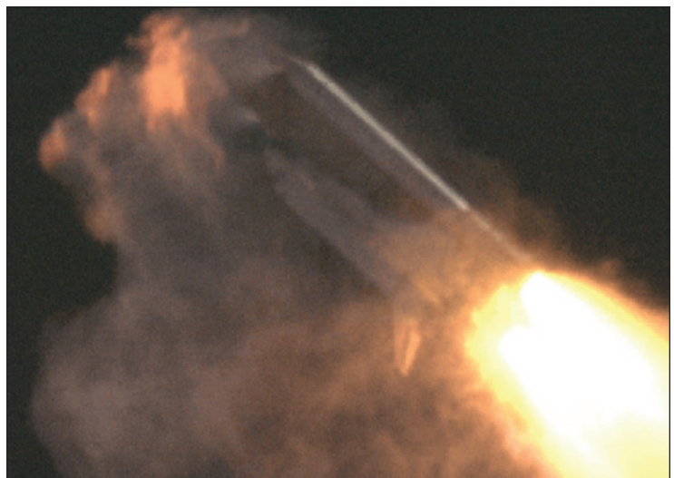
Figure 8: Shuttle ascent surrounded by Al_2O_3 smoke during BSM firing preceding booster separation
