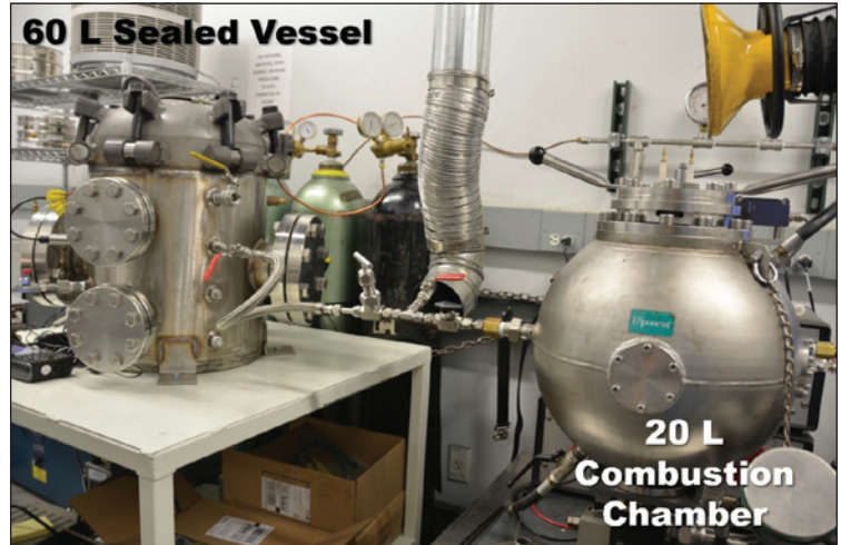
Figure 1: Photograph of a 60-liter sealed vessel connected to a 20-liter combustion chamber for battery vent gas explosion testing
