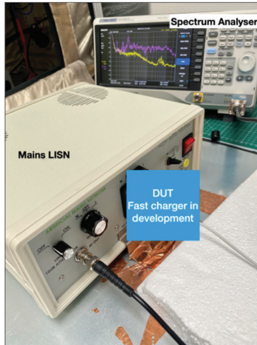
Figure 8: A fast charger is being tested against conducted emission in a pre-compliance test set-up
