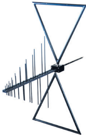
Figure 3: A typical full-sized calibrated EMI antenna. These can be 1m or more in size.
