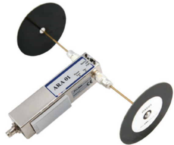
Figure 5: For a reduced-size calibrated antenna, I like an active antenna with built-in broadband RF preamplifier. This helps reduce the noise floor to compensate for the very short antenna elements.
