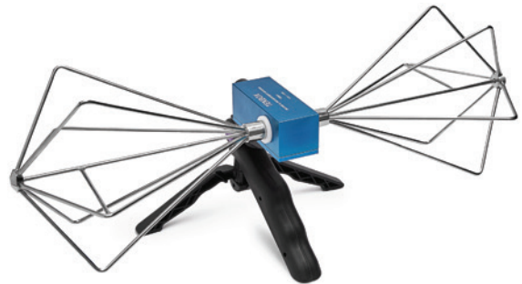
Figure 4: A physically small calibrated antenna that could work well at a 1m or 3m test distance. Because of the small dimensions, it would not be suitable at 10m.
