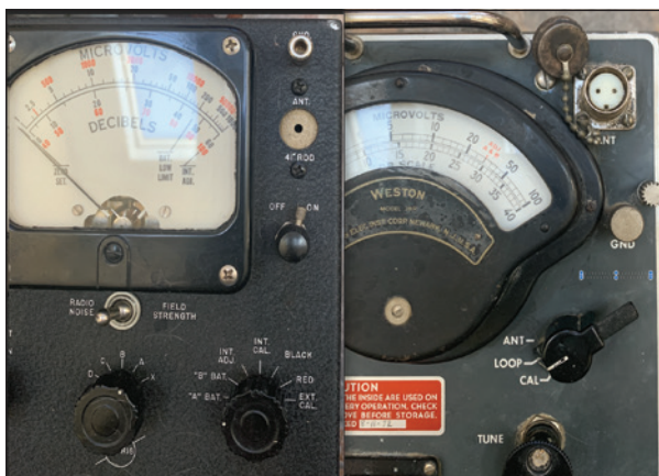
Figure 2a: Close-ups of rod antenna ports for the Ferris Model 32 on the left, and the Stoddart Aircraft Radio Company Model NM-20 on the right. Light-colored material surrounding the 1/8” diameter hole in the Ferris antenna port is a non-conductive standoff limiting shunt capacity to chassis. On the right, the two twinax pins are both connected to the rod element. The connector is not being used as twinax.
