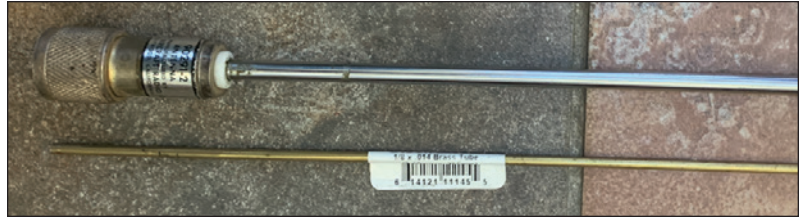
Figure 3: Stoddart Aircraft Company Model 90291-2 collapsible rod antenna assembly for use with NM-20 meter above, and 1/8" O.D. brass rod suitable for use with Ferris Model 32 meter below.
