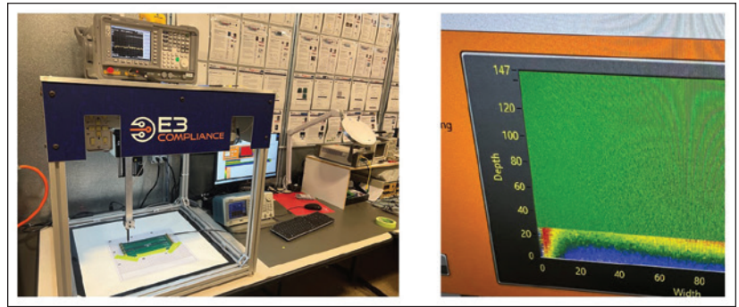
Figure 7: Experimental setup for frequency domain measurements
