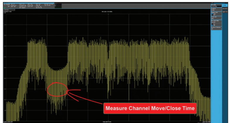
Figure 5: DFS channel move and close time FCC requirements for punctured 5 GHz channel
