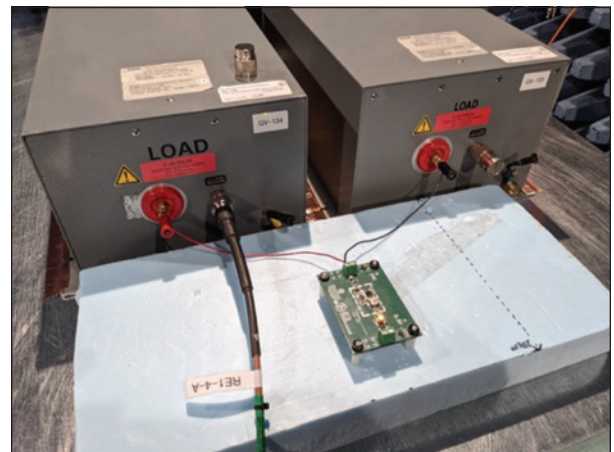
Figure 8: Conducted emission test setup (voltage method)
