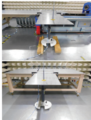
Figure 4: Measurement results comparing regular test table with EMC-BlueBox
