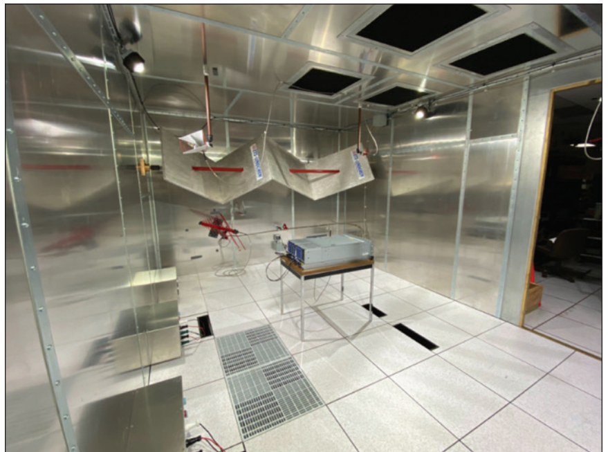
Figure 7: Shielding effectiveness testing in EMC reverb chamber
