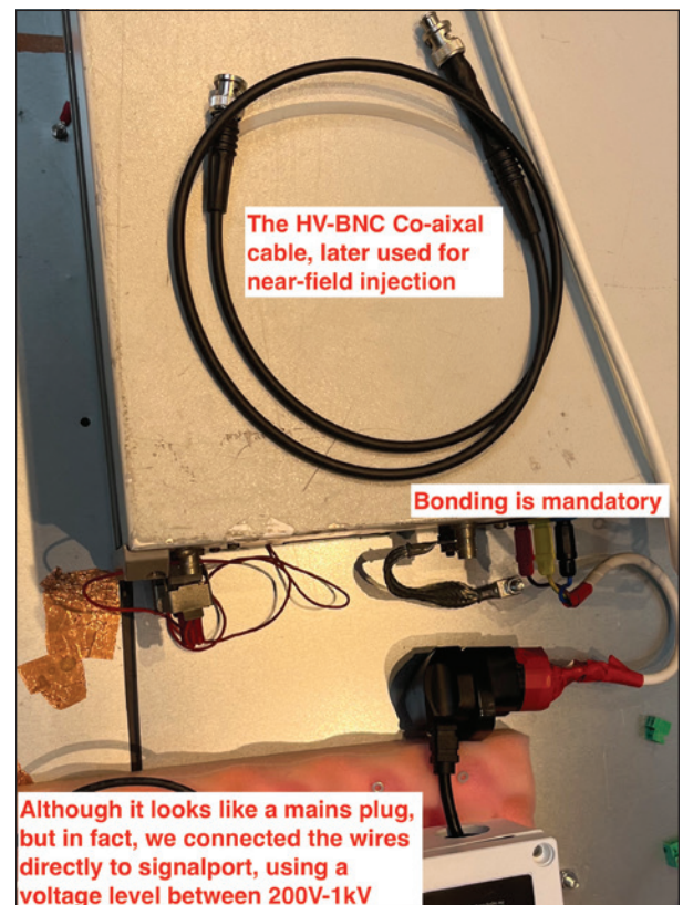
Figure 1: Using an EFT/Burst generator for troubleshooting
