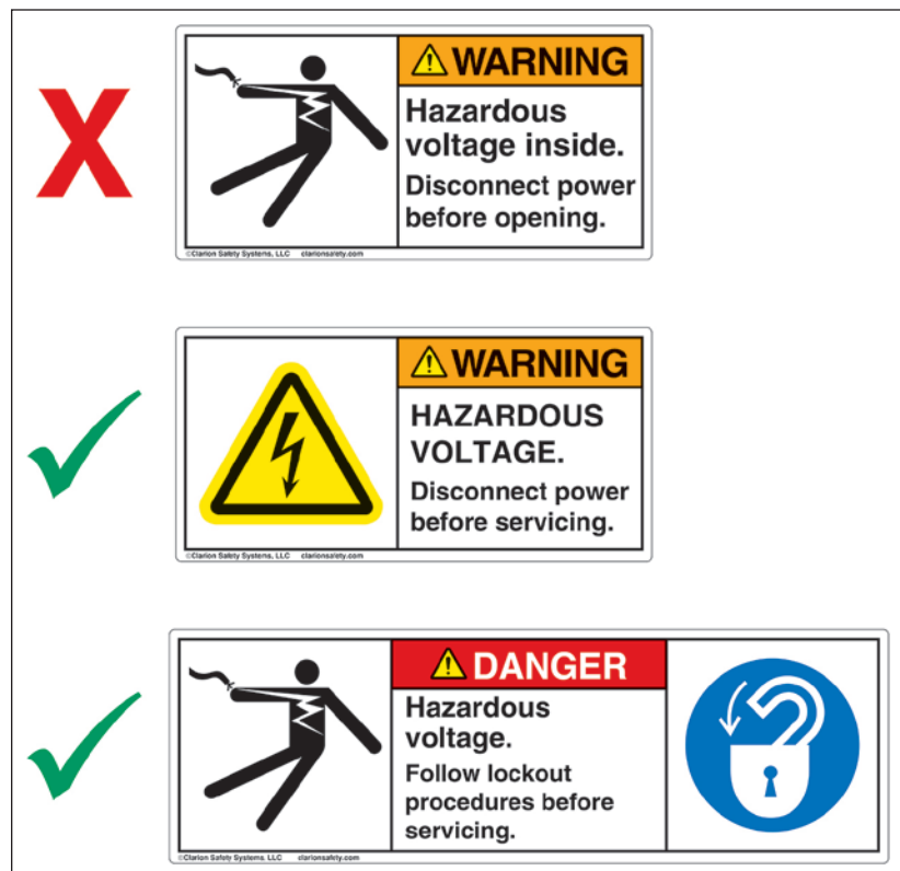
Figure 2: Examples of label formats that fail to comply (top) and comply (middle and bottom) with ISO 3864-2:2016. Per the standard, labels must use at least one ISO-formatted safety symbol in addition to the safety alert symbol in the label's severity level panel.
