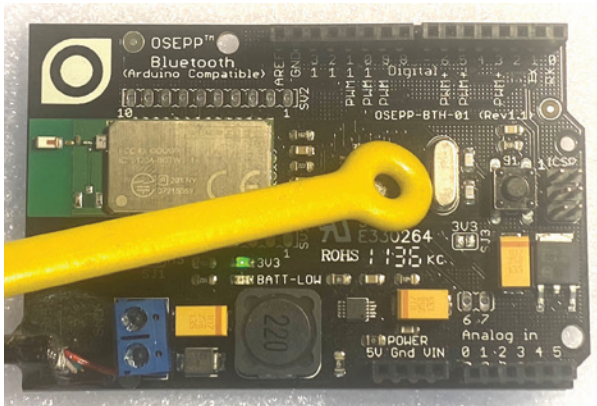
Figure 4: Using the medium-sized H-field probe to characterize the 16 MHz clock harmonics. These narrow band harmonics extend past 500 MHz.
