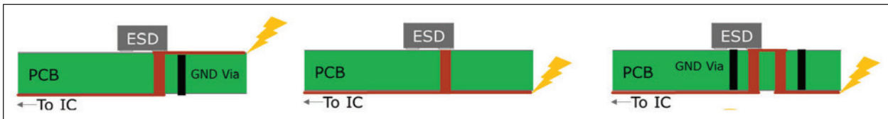
Figure 8: Routing options for changing layers. Try to route over the pad of the ESD device (left, right). Avoid via stubs (middle). Use adjacent ground vias when changing layers.
