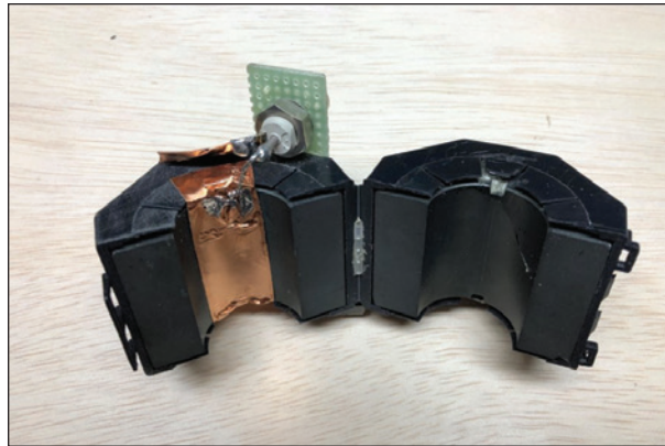
Figure 7a: DIY bulk current injection probe (single turn) for radiated immunity
