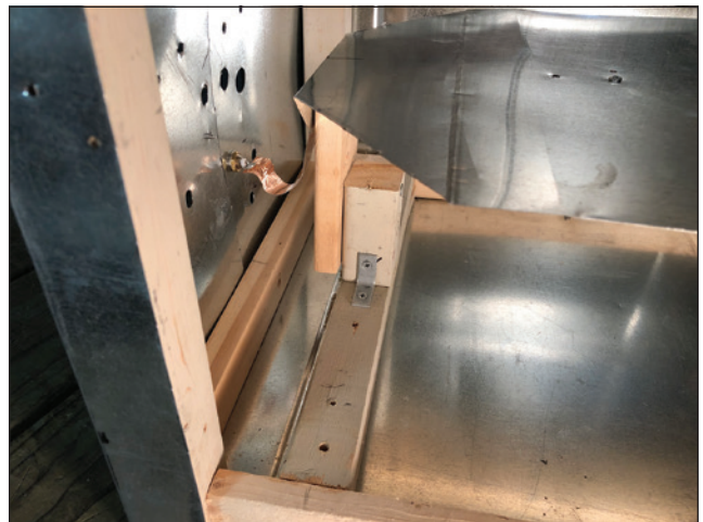
Figure 6c: TEM cell variant, end taper and BNC connection detail
