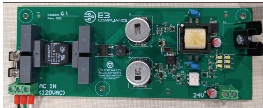
Figure 6: AC-DC converter PCB with components
