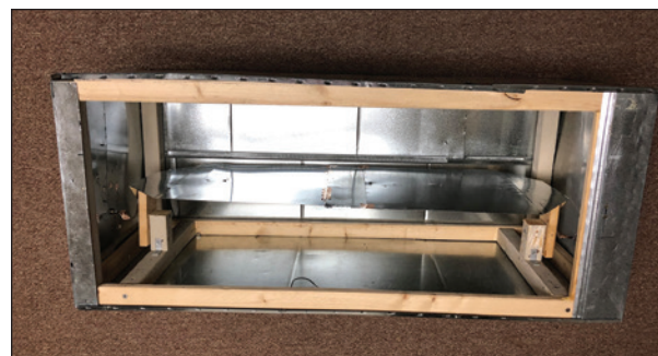
Figure 6a: DIY TEM cell variant (front door removed)
