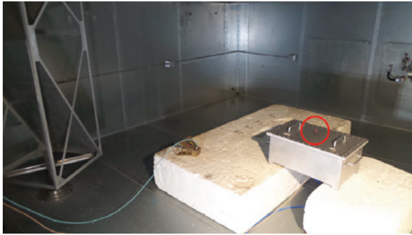
Figure 2: Nested cavity setup with N = 1 wire penetration
