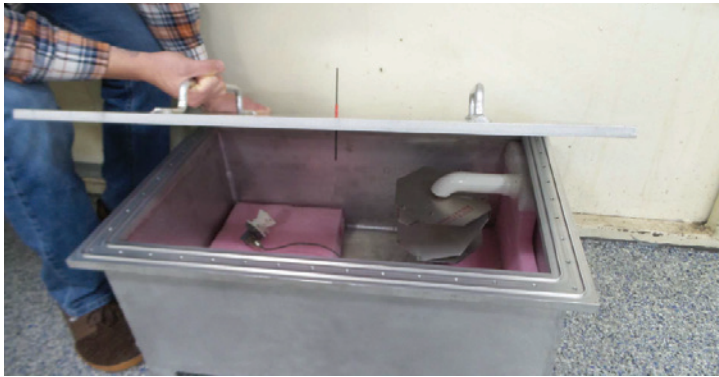
Figure 3: Nested enclosure setup with N = 1 wire penetration
