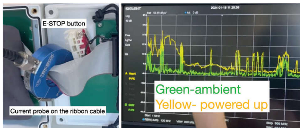
Figure 1: Measuring the RF common mode current on the ribbon cable
