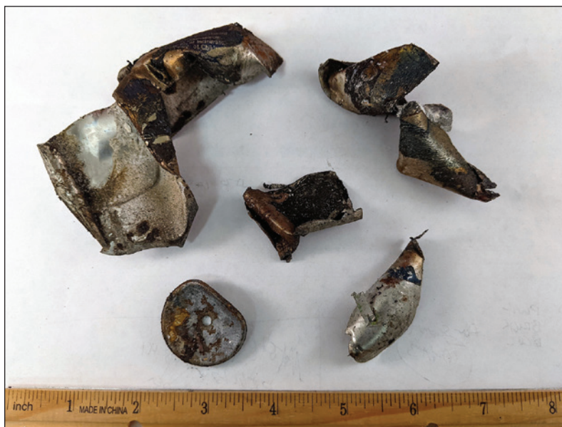
Figure 2: Lithium cell metal can fragment after thermal runaway
