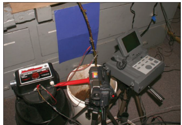
Figure 5: BullDozer single strand wire and potted blackberry test setup—also shown are a high voltage probe, a camcorder, and a thermal imaging camera
