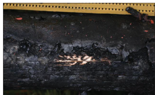
Figure 12: Incident Douglas fir tree trunk showing a Lichtenberg figure—the trunk was approximately 2 inches at this location, and the black marks at the top of the image is a scale in 16ths of an inch.
