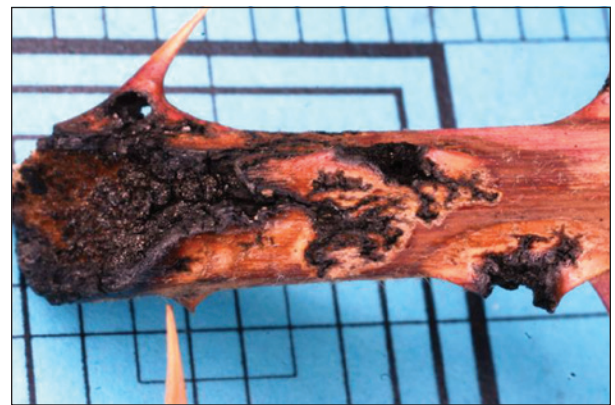
Figure 7: Lichtenberg figures in incident blackberry stalk
