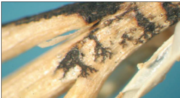
Figure 6: Lichtenberg figures in the incident wild mustard stalk
