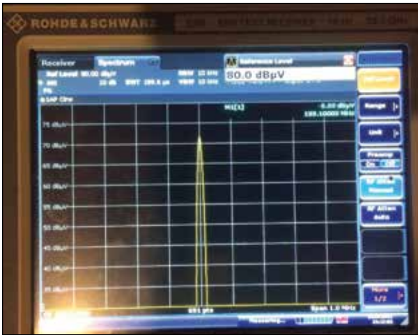
Figure 7a: Measured current with F-65 probe in place: dBuV = dBuA
