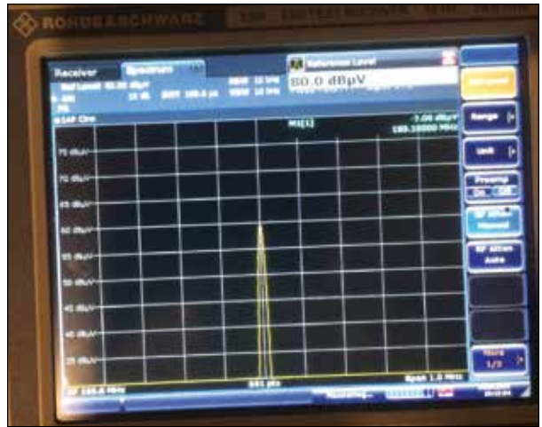
Figure 7b: Measured current with F-65 probe adjacent to Solar Model 9120-1N clamp: dBuV = dBuA
