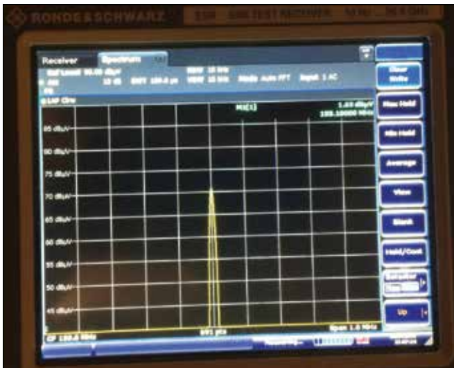
Figure 11b: Coupled potential when Model 9120-1N BCI clamp driven hard enough to induce 72 dBuA current on CUT.
