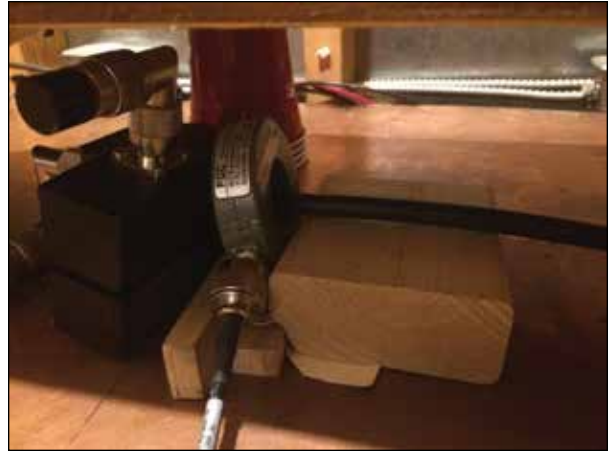
Figure 6b: FCC Model F-65 current probe with Solar Model 9120-1N to detune resonance
