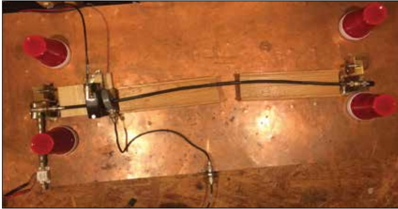
Figure 10: Overall view of the BCI set-up on the same cable that was illuminated under the plate. Solar Model 9120-1N on the left, FCC Model F-65 to its right.
