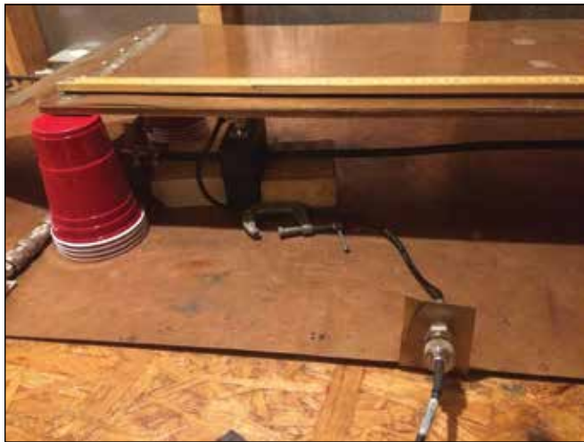
Figure 9a: Solar Model 9120-1N injection clamp used as current probe
