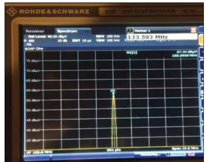
Figure 11d: Coupled potential when Model 9120-1N BCI clamp driven hard enough to induce 57 dBuA current on CUT.
