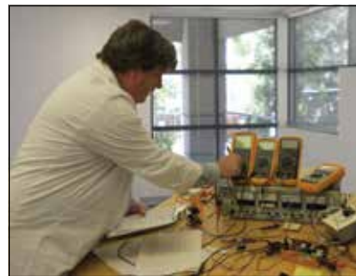
Meters testing: The lab staff are determining the energy levels available from a standard switch mode power supply with the goal of ensuring that the power available is limited to safe levels in accordance with the standard.
