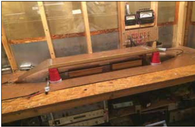
Figure 4a: CUT under plate. LNA connection visible at left.
