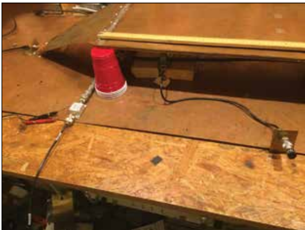
Figure 8a: Set-up for measuring potential coupled to RG-8 center conductor. In this figure, only the F-65 is placed under the plate.
