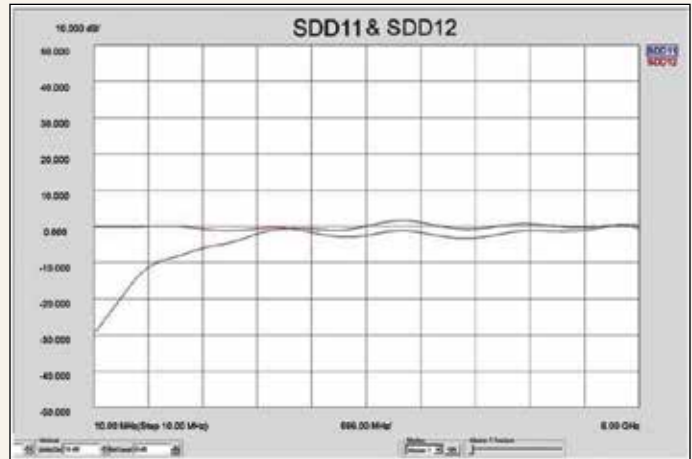
Test Data #1—Measured from 10 MHz to 6GHz (Note: SDD11 & 12 frequency domain RJ45 jack was de-embedded from test fixture.)
