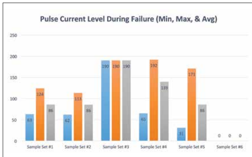
Figure 25: Minimum, maximum and average pulse current during failure for all tested diodes
