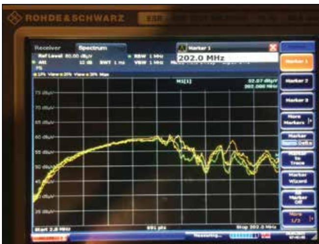
Figure 5: Core potentials (measured at output of LNA with 30 dB gain). All three traces are nearly coincident over most of the 2 – 200 MHz frequency range, but some differences are visible. The yellow trace is for no probe or clamp on the cable, the green trace is the F-65 around the cable, and the orange trace is with Solar Model 9120-1N clamped around the cable.
