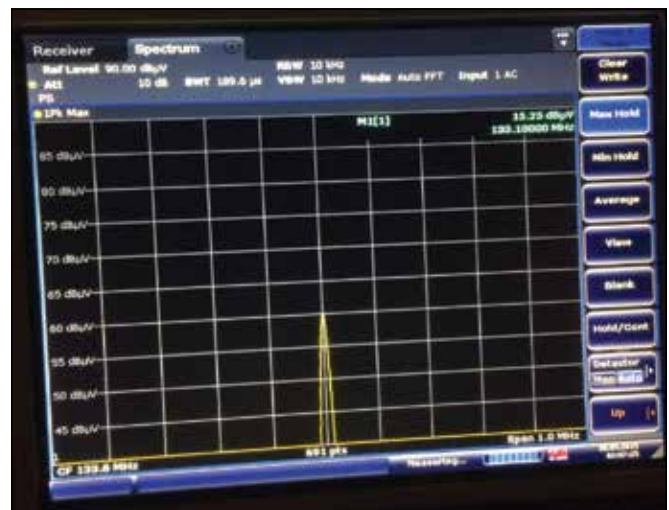
Figure 9c: Potential coupled to RG-8 center conductor when 57 dBuA current as per Figure 9b is induced on cable shield. 5 dB higher than measured in Figure 8b, which was coupled potential with the F-65 and also the Model 9120-1N around the cable.
