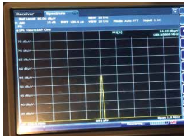
Figure 8b: Coupled potential (measured at output of 30 dB gain LNA) with and without the clamp in place. There are actually two separate traces here, but they are coincident, demonstrating that the placement of the high impedance clamp has no effect on the average cable-induced current.
