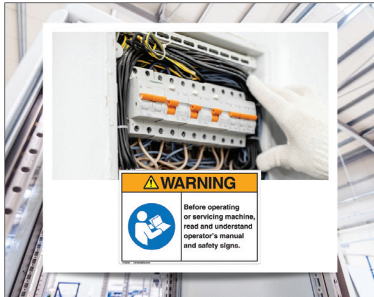
An example of a best practice, ANSI Z535-formatted ‘Read Manual’ safety label; the label includes the ISO 7010, internationally-standardized symbol for “Refer to instruction manual/booklet”.
