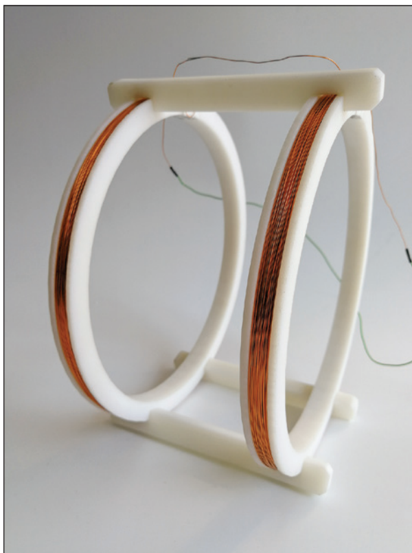
Figure 1: An example of a Helmholtz coil two-system for uniform magnetic field creation
