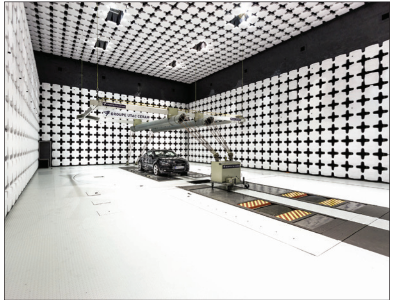
Figure 13: Automotive test chamber using polystyrene absorber (image courtesy of ETS-Lindgren)
