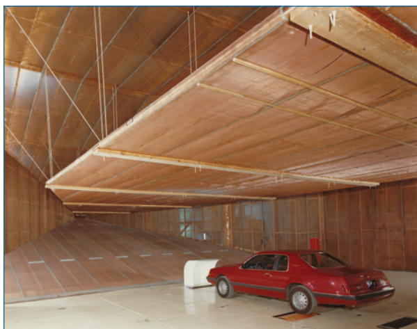
Figure 2a: Vehicle transverse electromagnetic (TEM) cell
