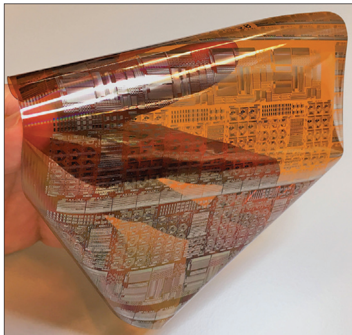
Figure 2: IGZO test circuits fabricated on a semi-transparent flexible substrate.
