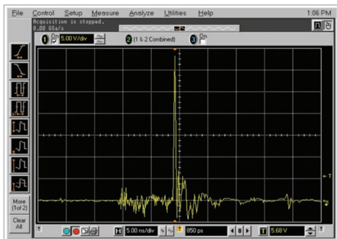
Figure 2: Example of ESD Induced Error in a Digital Oscilloscope (Vertical scale = 5 Volts/div, Horizontal scale = 5 ns/div)
