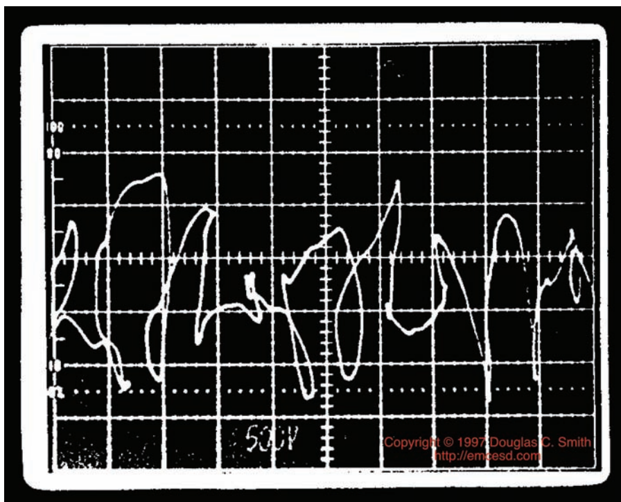
Figure 1: Example of ESD Induced Error in an Analog Oscilloscope
